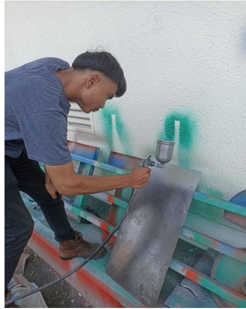
Proses pengecatan bodi
