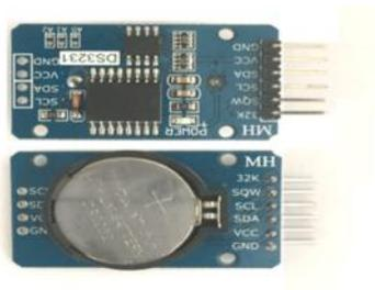
Gambar 4. RTC (Real Time Clock)
