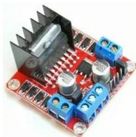
Gambar 10. Driver Motor Modul
