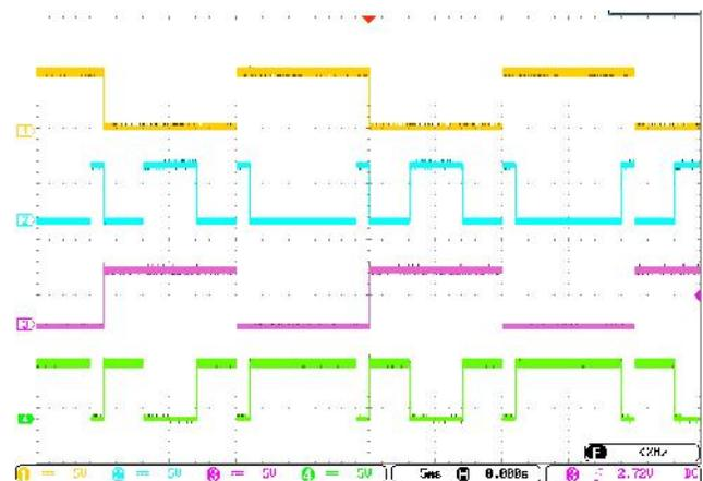
Fig. 4: Switching angles S<sub>1a</sub>–S<sub>4a</sub> for  $m_a=0.84$ ,  $\alpha_1=17.06^\circ$ ,
