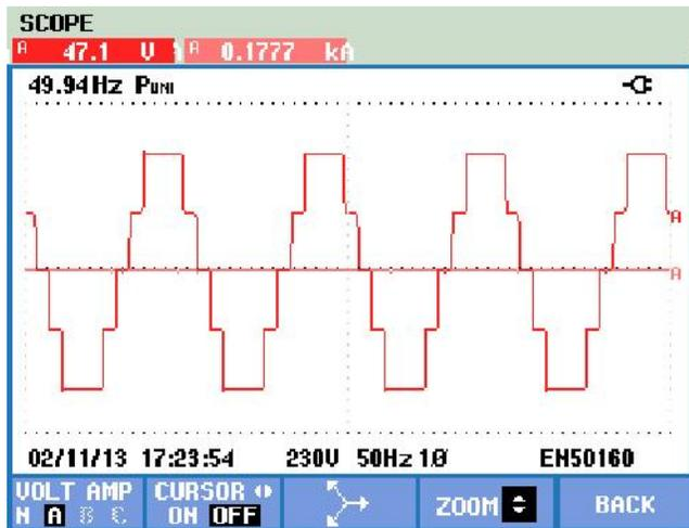
Fig. 6: Output voltage  $m_a=0.84$ ,  $\alpha_1=17.06^\circ$ ,  $\alpha_2=43.53^\circ$
