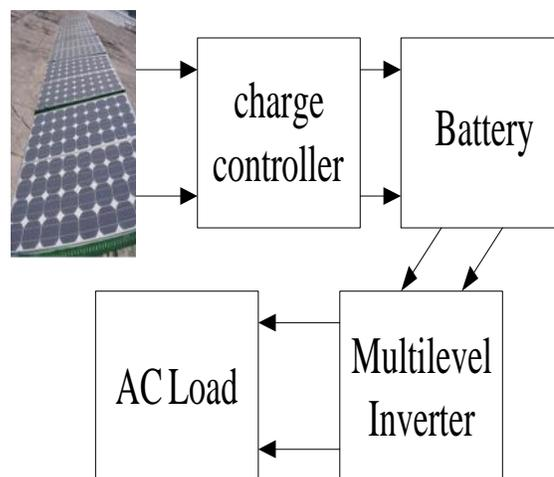
Fig. 1. Photovoltaic inverter configuration
