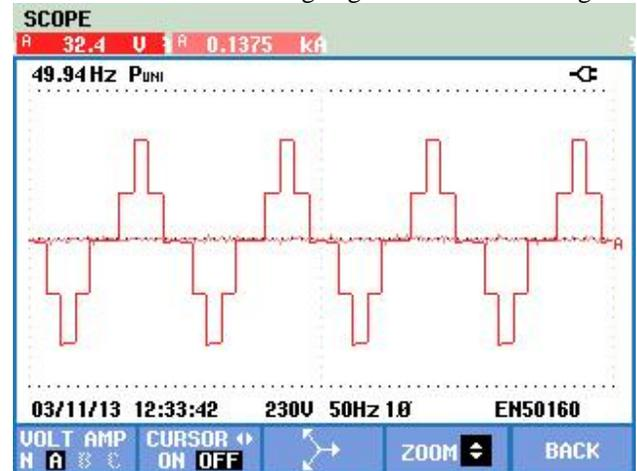
Fig. 8: Output voltage  $\alpha_1=30^\circ$ , and  $\alpha_2=75^\circ$
