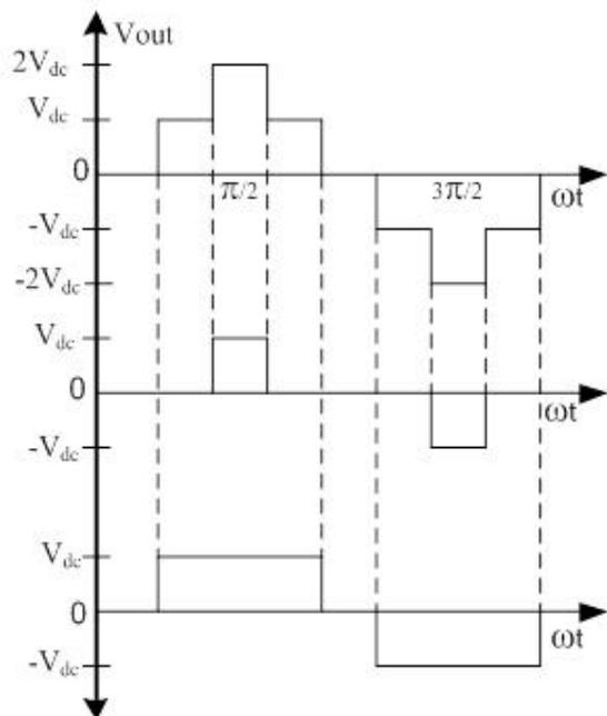
Fig 3. Output Voltage of CHB five level inverter
