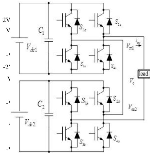
Fig. 2. The single-phase CHB multilevel inverter
