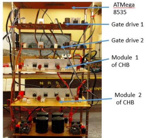
Fig. 10: Hardware setup
