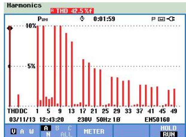
Fig. 9: Harmonic content output current waveform  $\alpha_1=30^\circ$ ,  $\alpha_2=75^\circ$ ,
