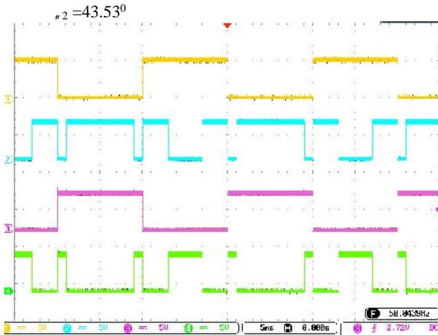
Fig.5: Switching angles  $S_{1b}$ - $S_{4b}$  for  $m_a=0.84$ ,  $\alpha_1=17.06^\circ$ ,  $\alpha_2=43.53^\circ$
