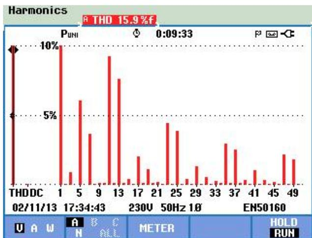
Fig. 7: Harmonic content output voltage waveform for  $m_a=0.84$ ,  $\alpha_1=17.06^\circ$ ,  $\alpha_2=43.53^\circ$
