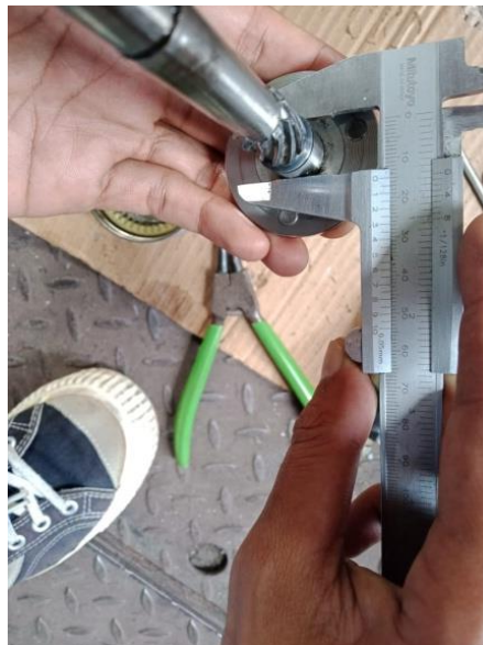
Gambar 38. Periksa Poros Planet Carrier dan Center Bearing
