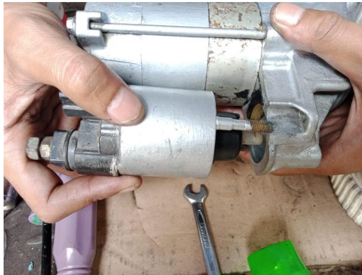
Gambar 47. Pasang Magnetic Switch
