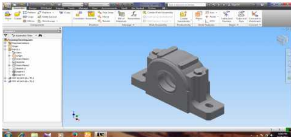
Gambar 4.32. Bearing take up station
