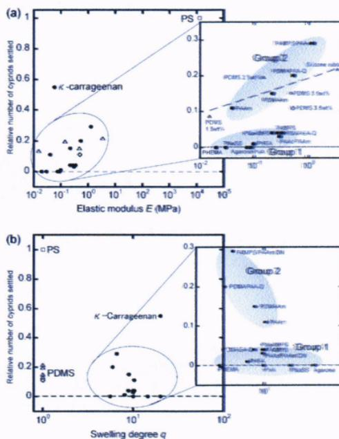
Figure 5. The relationship between the numbers of cyprids settled on the bottoms of wells after 5 days exposure and the (a) elastic modulus, and (b) swelling degree of bottom materials.  $\bullet$  = hydrogels;  $\diamond$  = PDMS (first run);  $\Delta$  = silicone elastomer (PDMS) with different elastic moduli;  $\square$  = PS.
