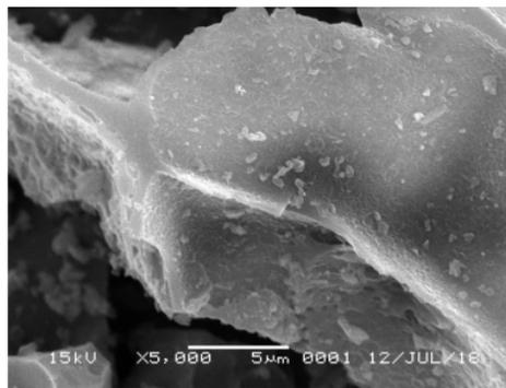
Fig. 9. The scanning electron microscopy (SEM) image of non-activated carbon of the palm shell with a magnification of 5000x
