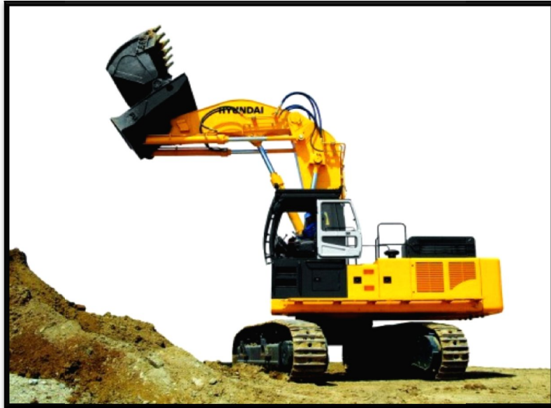
Gambar 9. Excavator Jenis Power shovel
