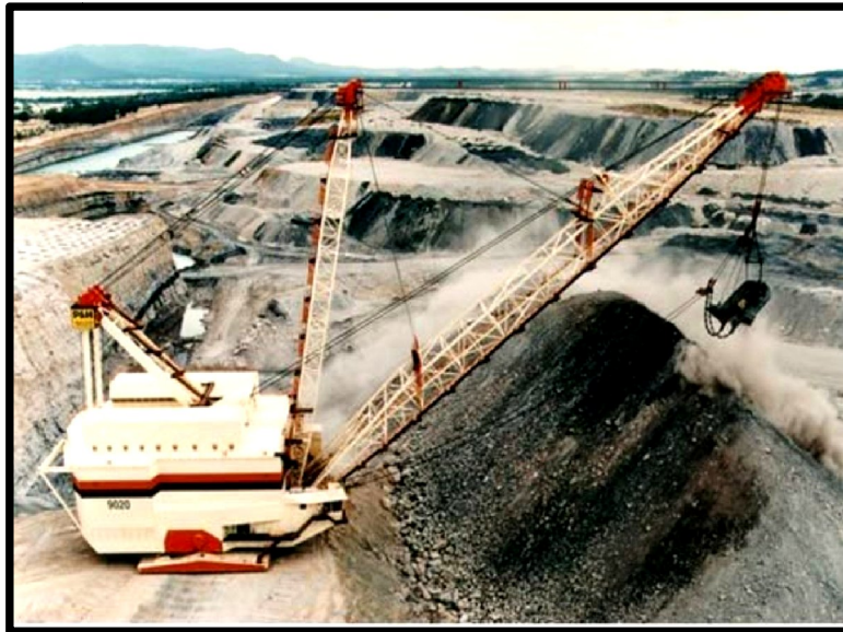
Gambar 8. Excavator Jenis Dragline
