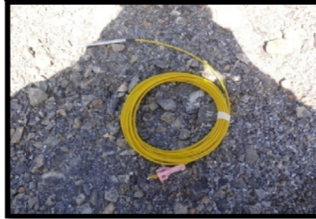
Gambar 12. Detonator nonel ( non electric )
