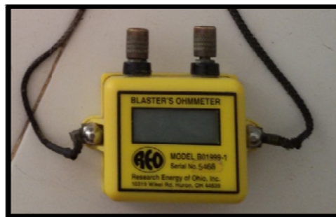
Gambar 8. Blasting Ohm Machine (BOM)
