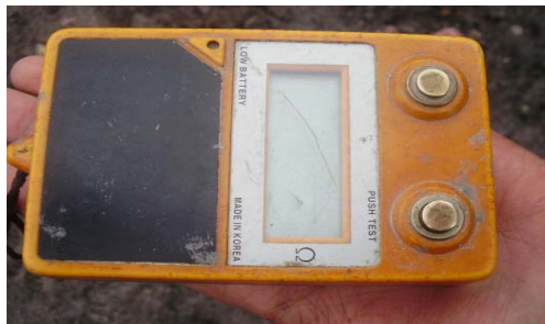
Gambar16: Blasting ohm meter
