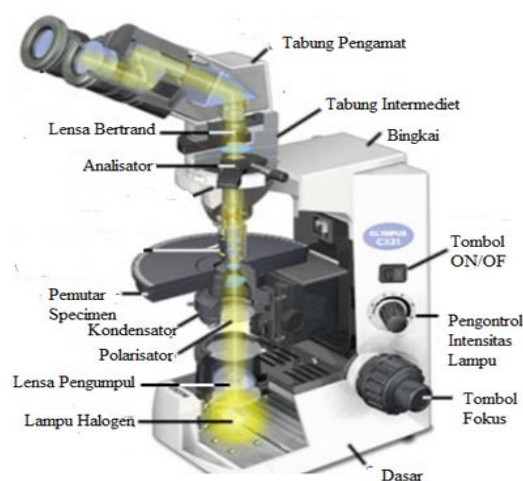
Gambar 18. OPM ( Optical Polarizing Microscop )
