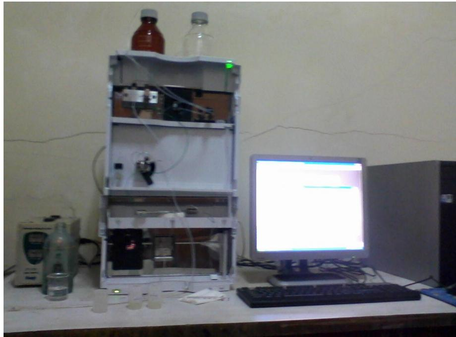
Gambar.3 HPLC (*High Performance Liquid Chromatography*)
