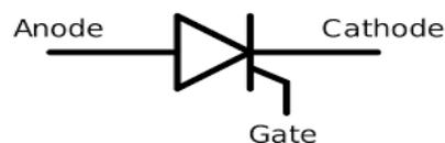
Gambar 7. Simbol Silicon Controller Rectifier (SCR)
