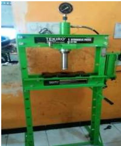
**Gambar 2.** Alat Press Hidrolik
