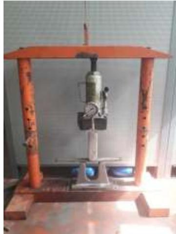
**Gambar 1.**Alat Uji *Bending* di Workshop Teknik Mesin FT UNP
