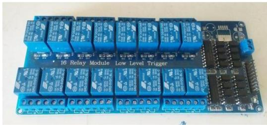
Gambar 6. Modul Relay 16 Channel
