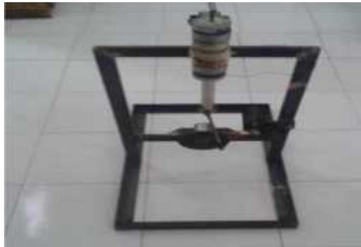
Gambar 11. Desain Prototipe *Electromagnetic Regenerative Shock Absorber*
