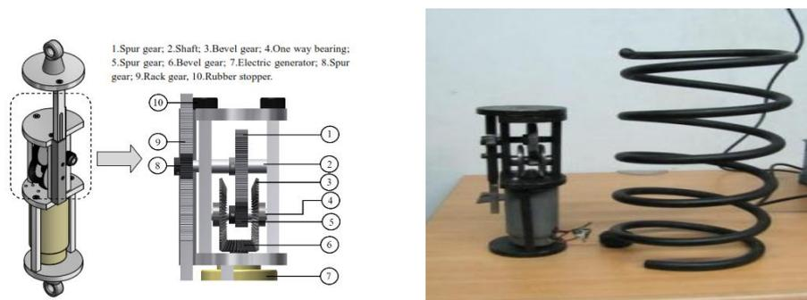
Gambar 16. *Desain regenerative Shock Absorber*
