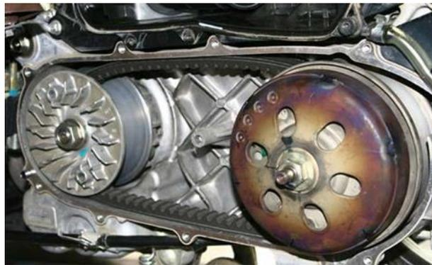
Gambar 1. CVT (*Continuously Variable Transmission*)
