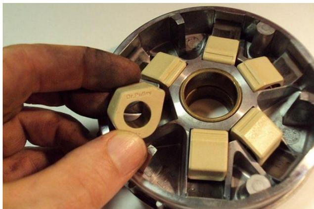
Gambar 3. Roller Tipe Sliding
