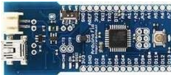
Gambar 6. Arduino Fio Sumber : Feri Djuandi (2011)
