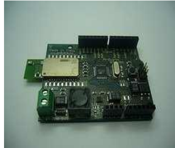
Gambar 8. Arduino BT Sumber : Feri Djuandi (2011)
