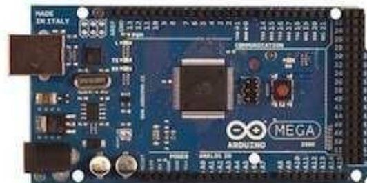
Gambar 5. Arduino Mega Sumber : Feri Djuandi (2011)
