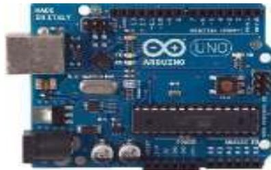
Gambar 4. Board Arduino Uno
