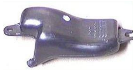
Gambar 4. Tabung Induksi Sumber: SAE (Society of Automotive Engineering), Inc.
