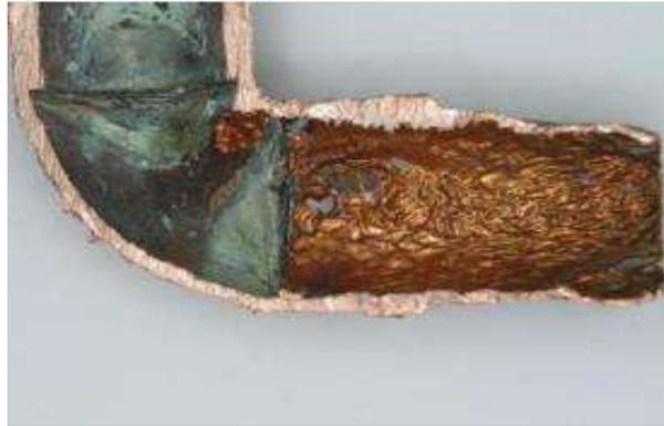
Gambar 5. *Errosion Corrosion* (Utomo, 2009)
