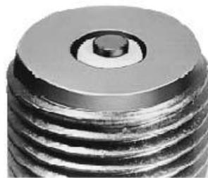
Gambar 10. Busi Semi-Surface Discharge
