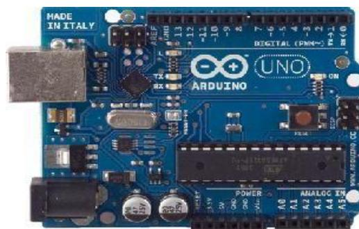
Gambar 7. Board Arduino Uno
