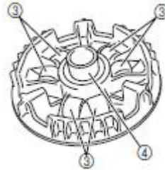
Gambar 6. Roller CVT pada *Movable Drive Face/Primary Sliding Sheave* (Sumber : Yamaha Motor Co., Ltd. : Service Manual Mio, 2003)
