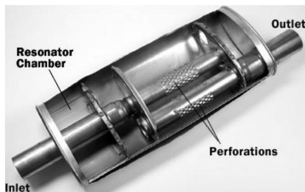
Gambar 9. Muffler standar
