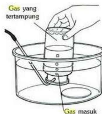
Gambar 12. Mengukur Volume Gas
