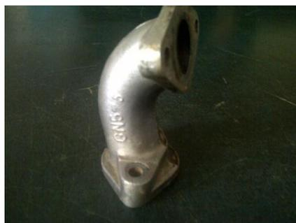
**Gambar 2.** *Intake Manifold* Standar
