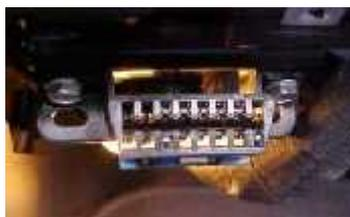
Gambar 16. Contoh DLC ( Data Link Connector )
