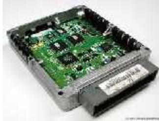
Gambar 7. Contoh ( ECU ) Engine Control Unit
