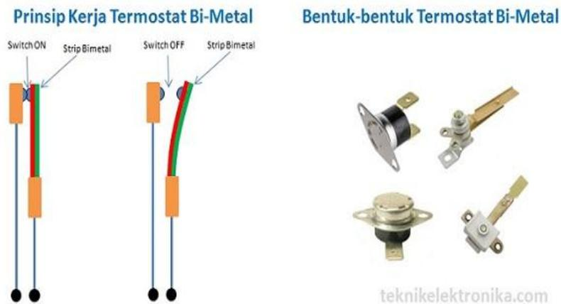
*Gambar 7. thermostat mekanik
