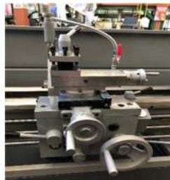
Gambar 2. 6 *Carriage* (Eretan Mesin Bubut)
