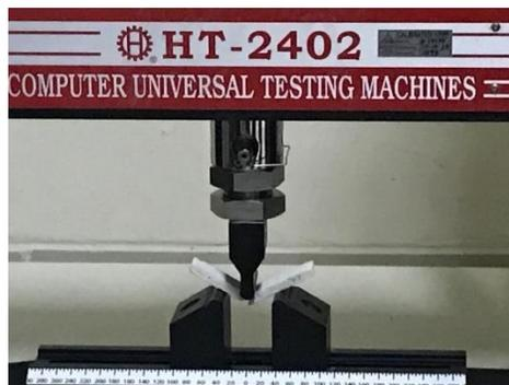
**Gambar 10. Bending Testing Machine**
