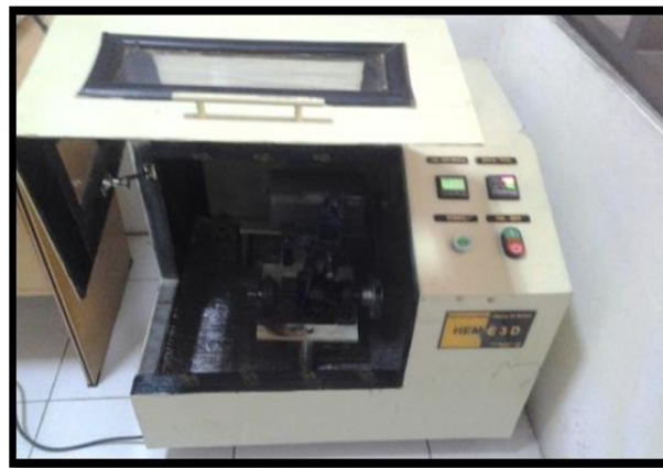
Gambar 9. High Energy Milling Ellipse 3D (HEM-E 3D)
