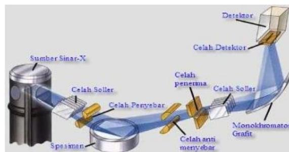
Gambar 6. Skema kerja instrumen XRD (Wardani, 2010)
