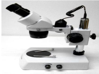
Gambar 2.9 Mikroskop Stereo (Hale, 2007)
