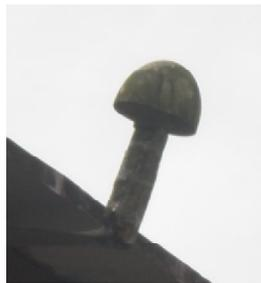
Gambar 10. Antena GPS
