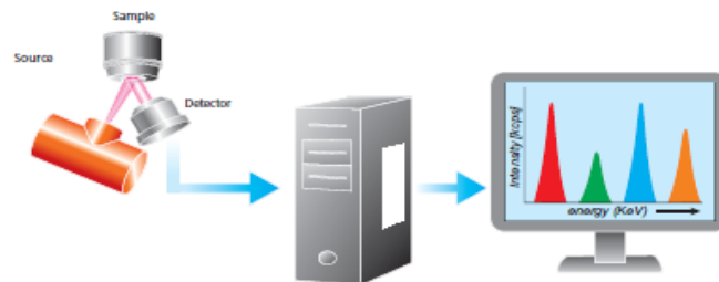
Gambar 7. Prinsip Kerja EDXRF (Brouwer, 2010).
