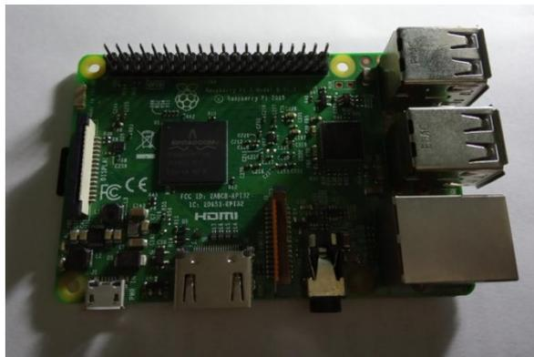
Gambar 5. *Raspberry Pi 3 Model B*
