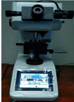
**Gambar 7. Alat Vickers Hardness Tester**
