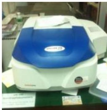
Gambar 17. Spektrofotometer UV-VIS (Laboratorium Kimia UNP)
