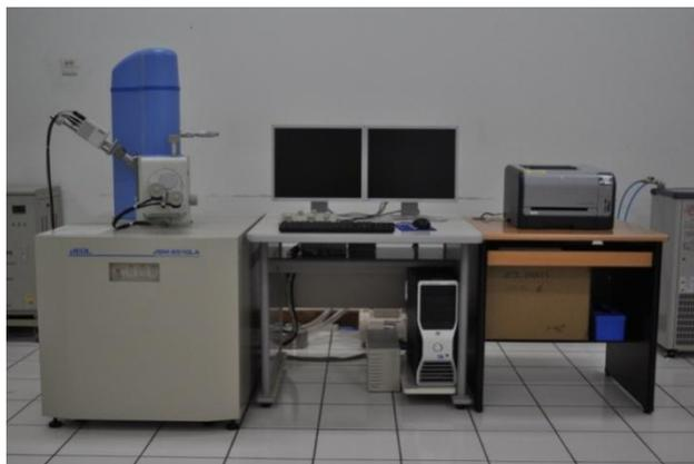
Gambar 15. Alat SEM tipe JEOL-JSM-6510 LA (Sumber: Laboratorium SEM FMIPA ITB)
