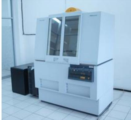
Gambar 13. XRD tipe X'Pert Powder PW 30/40
