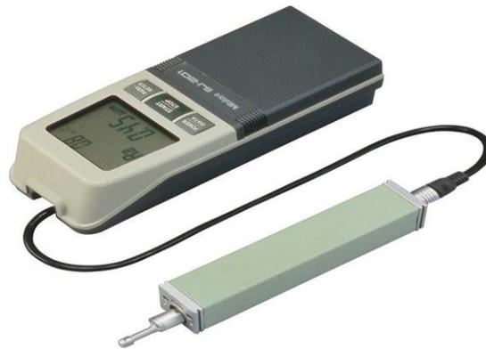
Gambar 18. Surface Roughness Tester SJ-201P Mitutoyo
