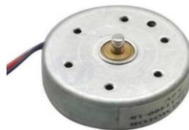
Gambar 12 Motor DC 9V
