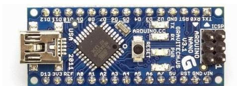
Gambar 10. Board Arduino Nano Tipe R3
