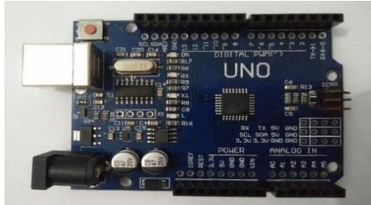
Gambar 3. Board Arduino Uno
