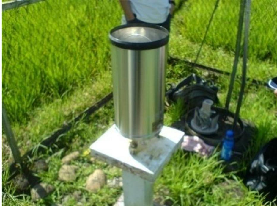
Gambar 8. Pengukur Hujan Otomatis (ARG/Automatic Rain Gauge)
