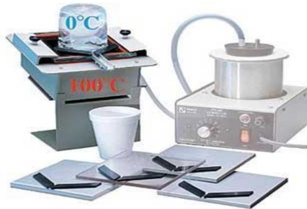
Gambar 5. Thermal Conductivity Apparatus
