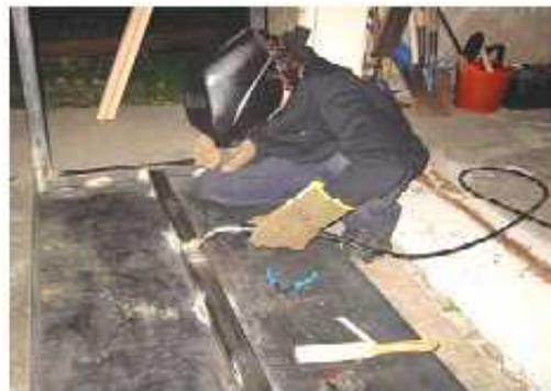
**Gambar 31.** Operasional Las MIG (*Metal Inert Gas*)
