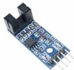
Gambar 5. Sensor *Optocoupler*
