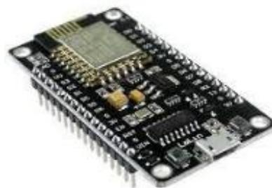
Gambar 4. *Board* NodeMCU ESP8266
